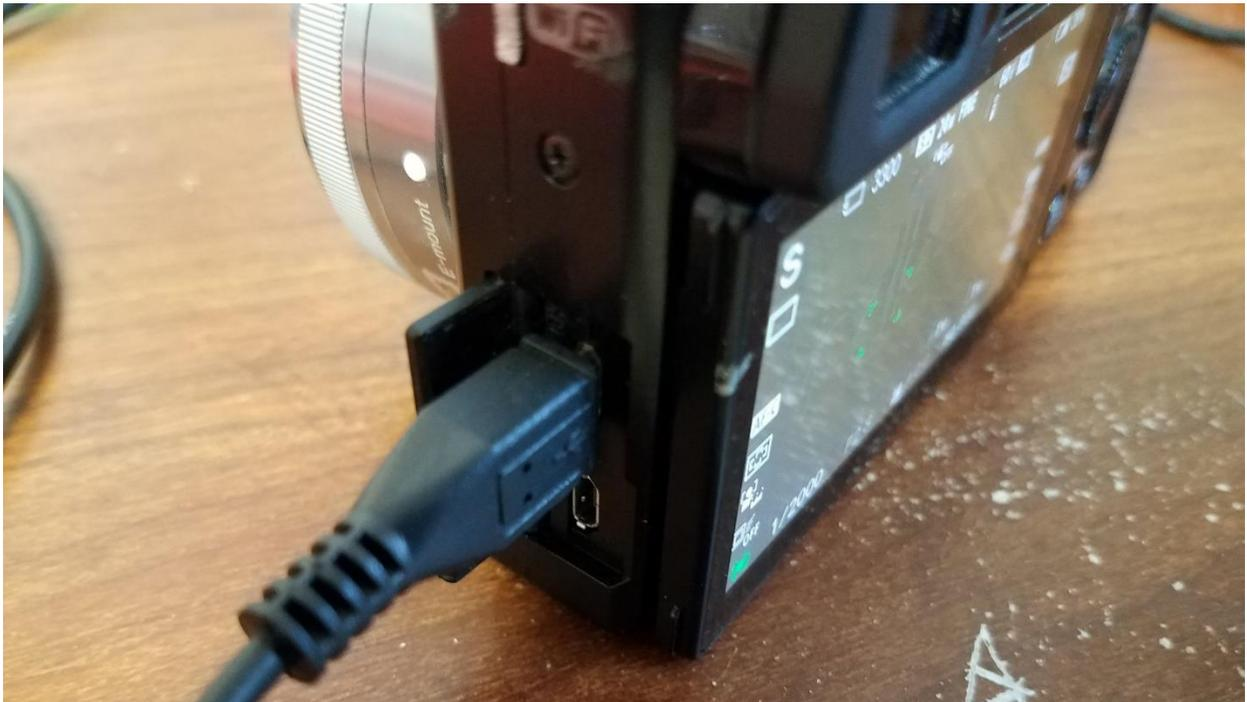
Since we have shorted the FOCUS and GROUND wires, the camera should automatically pull focus. As of now, I have not found a way to connect the SHUTTER, FOCUS and GROUND wires individually to the Pixhawk/APM and have the flight controller pull the camera focus and trigger the camera in sequence. To get around this, the camera settings are set so that the camera has the following features activated:
