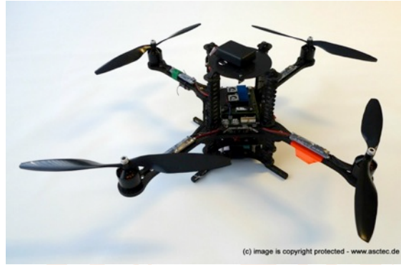
AscTec Pelican (unloaded) ( m = 964\text{g} )
